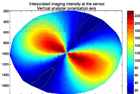
Figure 5: Interpolated imaging intensity for a panomorph lens. The polarization axis of the analyzer is vertical.
