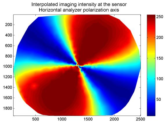
Figure 6: Interpolated imaging intensity for a fisheye lens. The polarization axis of the analyzer is horizontal.
