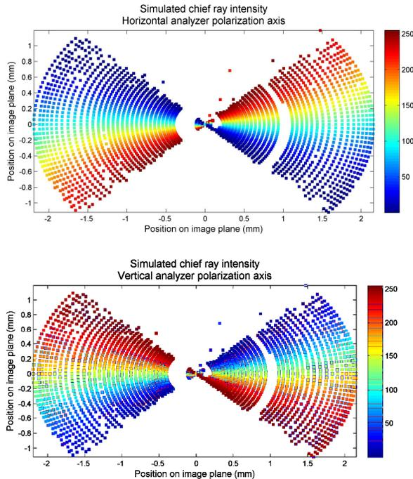
Figure 8: Simulated results for the panomorph lens with the analyzer horizontal (top) and vertical (bottom) polarization axis.
