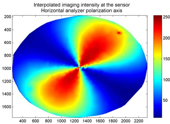
Figure 4: Interpolated imaging intensity for a panomorph lens. The polarization axis of the analyzer is horizontal.
