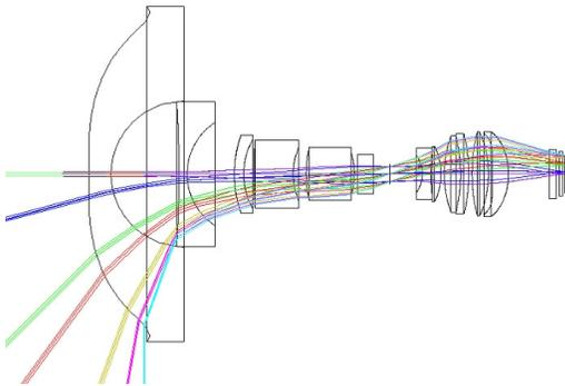
Figure 2: Layout of a typical panomorph lens
