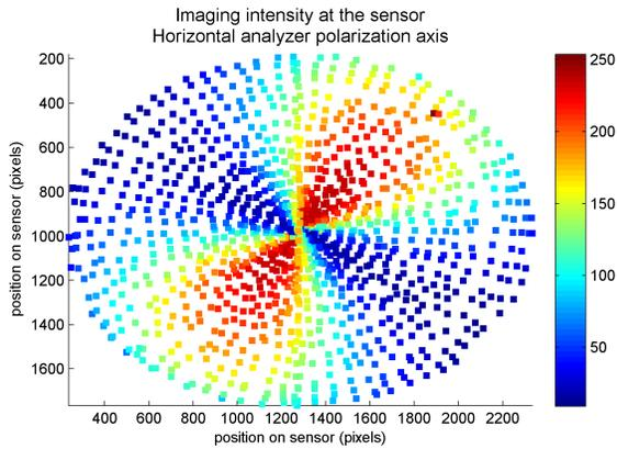
Figure 3: Measured intensities averaged on a 10X10 pixels zone of a panomorph lens. The polarization axis of the analyzer is horizontal.
