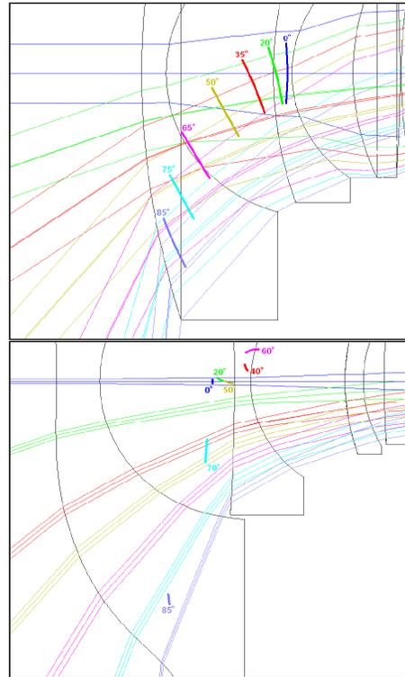
Figure 9: Entrance pupil displacement at various fields of views for a standard wide-angle fisheye lens (top) and the Panomorph lens (bottom).
