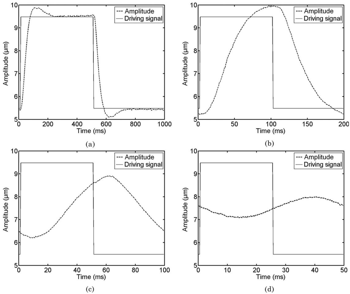
Fig. 3. Amplitude response of a ferrofluid having a viscosity of 6 cP driven by a single actuator using square waves of (a) 1 Hz, (b) 5 Hz, (c) 10 Hz, (d) 20 Hz.
