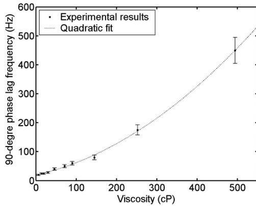
Fig. 4. Frequency at which a 90° phase lag is reached as a function of ferrofluid viscosity. The dashed curve shows a quadratic fit to the results.
