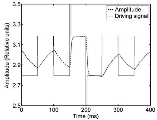
Fig. 5. Effect of adding short pulses at the beginning of the step signals to counter the amplitude loss. When overdriving is used, this ferrofluid of 90 cP viscosity demonstrates a good response with waves of 10 Hz (correction frequency of 20 Hz). We can also note that the phase lag is negligible at this frequency as opposed to Fig. 3(c), in which the viscosity of 6 cP produced a clearly visible phase lag.
