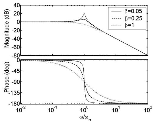
Fig. 1. Example of Bode diagrams for a classical damped harmonic oscillator.
