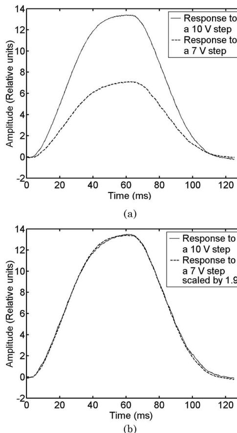
Fig. 2. Ferrofluid response to two step functions having different amplitudes. (a) Raw measurements for both curves. (b) The dashed curve is scaled to match the second.
