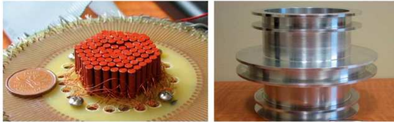
Fig. 2. Pictures of the 91-actuator FDM (left) and Maxwell coil (right). The Maxwell coil is shown prior to winding. The three winding areas of Fig. 1 can clearly be seen.
