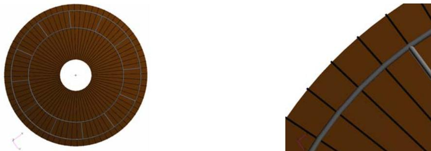
**Figure 2-4: Rib sections supporting mirror surface panels**
