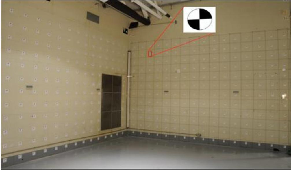
***Figure 4: 339 targets of calibration object***
