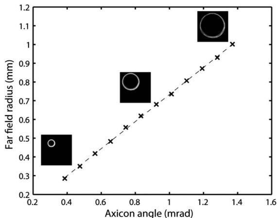
Fig. 6. Measured radius of the annular far-field beam as a function of the different axicon cone angles produced by the MLDM through a linear scaling of the currents that were used to produce a 0.5 mrad axicon cone angle. The values of the angles are computed from the surface maps recorded by the WFS.
