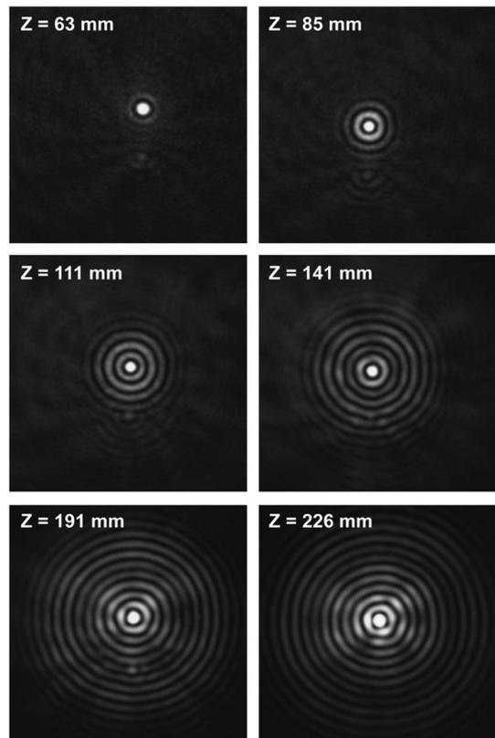
Fig. 2. Evolution of the spatial profile of the Bessel beam produced by a 0.50 mrad MLDM axicon along the propagation axis and recorded with the CMOS camera. Each image has a size of 1.56 mm  $\times$  1.56 mm.
