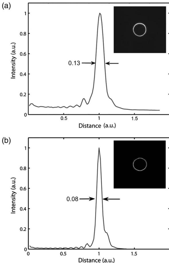
Fig. 5. (a) Observed far field produced by a 0.50 mrad MLDM axicon and imaged on the CMOS camera by a 300 mm focal length lens (insert). (b) Computed far-field distribution and simulated image (insert) using the Fourier transform of the conical surface recorded by the WFS. Both plots show a radial mean of the intensity distribution. The FWHM of the rings is given in relative units of the ring radius.
