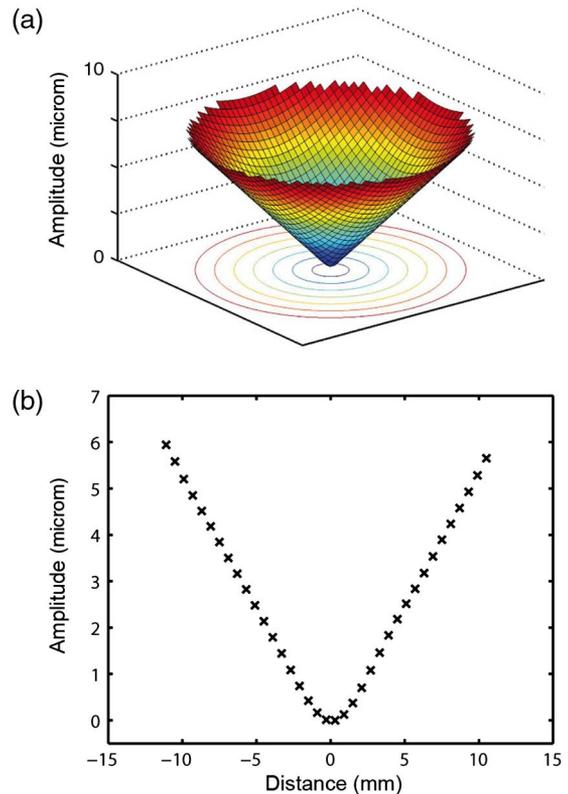
Fig. 4. (Color online) (a) Surface of a  $0.5$  mrad axicon produced by the MLDM and recorded by the WFS. (b) Plane cut of (a) showing the cone tip.
