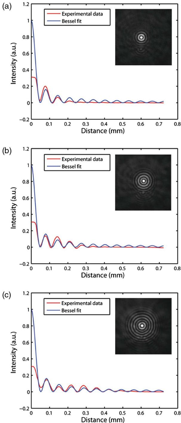
Fig. 3. (Color online) Mean radial intensity of the measured beam profile at three positions along the propagation axis ( $z = 85, 111,$  and  $151$  mm) and fitted using the same Bessel beam profile.
