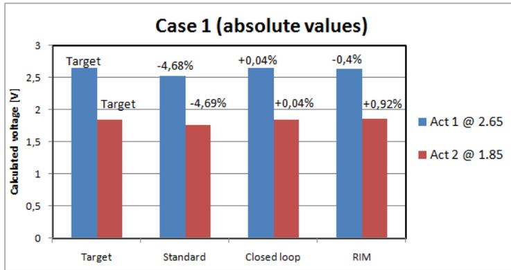
Figure 2: Comparison of the different input voltage measured using three different techniques; standard calculation, closed-loop and RIM for case 1 defined in text.
