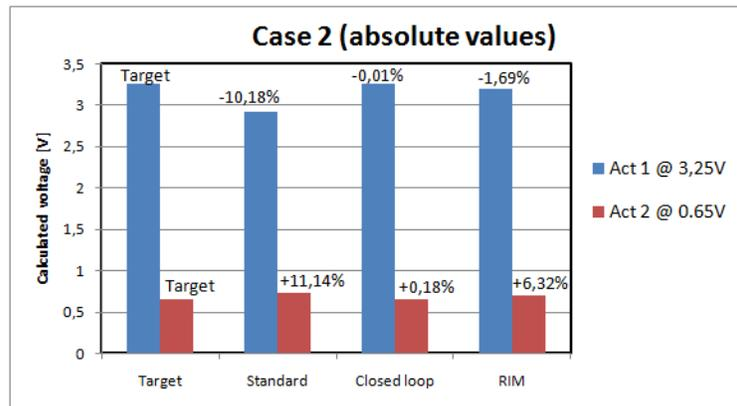
Figure 3: Comparison of the different input voltage measured using three different techniques; standard calculation, closed-loop and RIM for case 2 defined in text.
