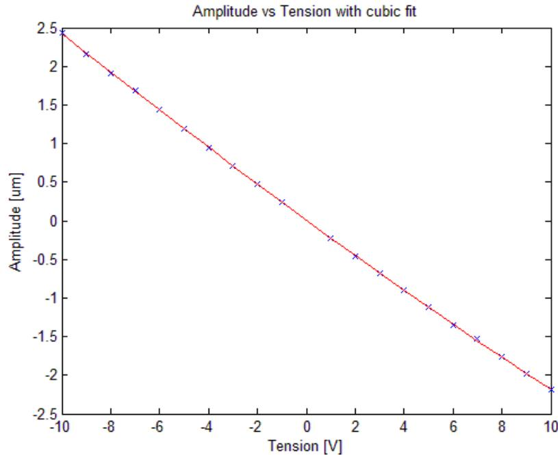
Figure 1: a) Linear fit for one pixel of the wavefront measured with voltages ranging from -10V to +10V.  $R^2=0.9993$  by equation  $y=-0.2309x+0.05034$ . b) Linear fit of the same data.  $R^2=0.9981$  by the equation  $y=-0.2319x$ . c) Cubic fit of the same data.  $R^2=1$  by the equation  $y= 1.463e-005x^3+0.001136x^2-0.2319x+ 0.006585$ .
