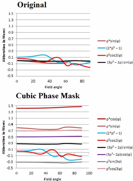
Fig. 2 Zernike aberrations as a function of the field for the original system and the system with a cubic phase mask. The phase mask adds various aberrations but they are almost independent on the field of view.
