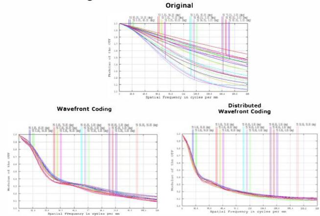
Fig. 3 MTF of the original and modified system.
