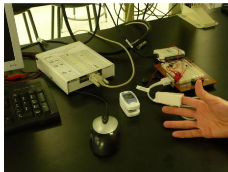
**Figure 5.** Oxymeter set-up as installed in an undergraduate teaching laboratory
