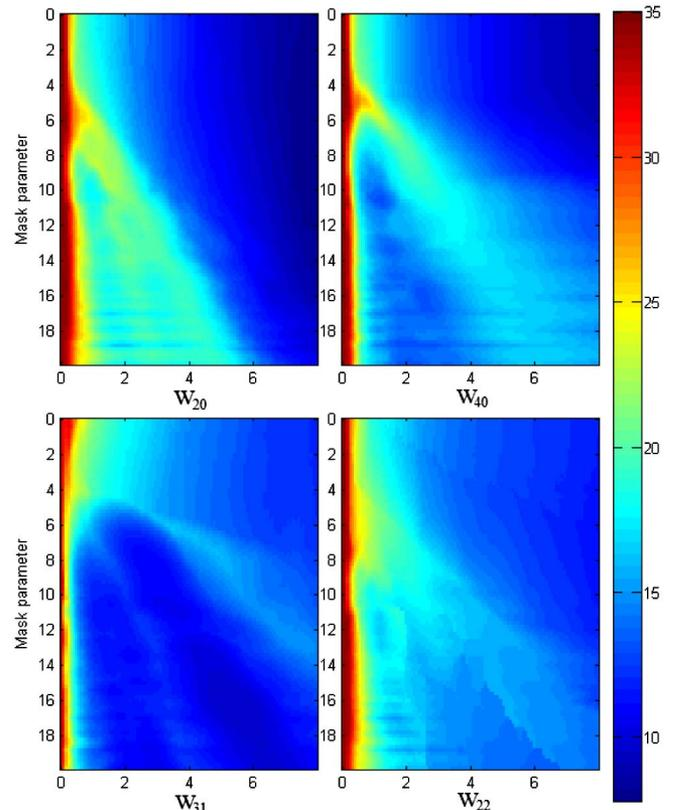
Fig. 1. RIQ as a function of aberration and cubic phase-mask parameter. No noise is added.
