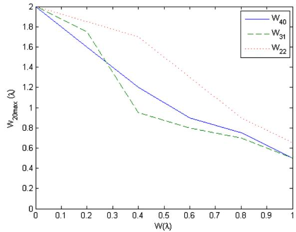
Fig. 3. Maximum compensated defocus as a function of the aberration coefficient for spherical, coma, and astigmatism.
