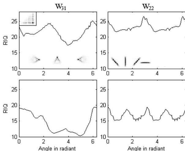
Fig. 2. RIQ as a function of the relative angle of the PSF for astigmatism and coma. The first row presents data for a phase-mask parameter  $\alpha = 5$  and  $1\lambda$  of aberration. In the second row,  $\alpha = 15$  and the aberration is  $3\lambda$ .
