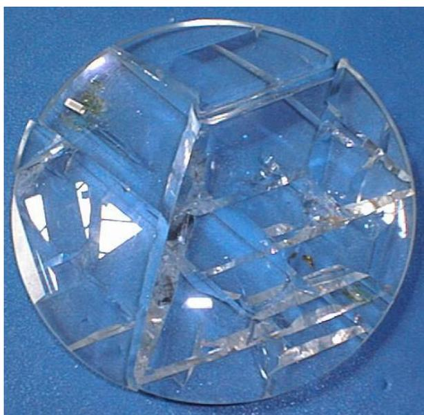
Figure 1: BaF<sub>2</sub> lens brakes during a cooling in 40 mn[2]
