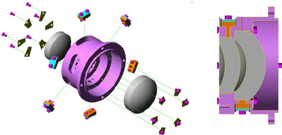
Figure 5: Explode view of GPI lens mount.
