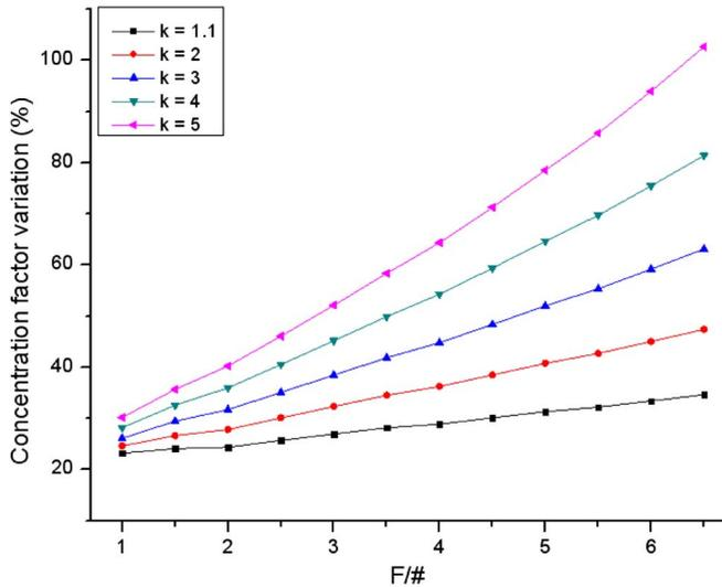
Fig. 3. Variation of the concentration factor associated with the use of a GRIN waveguide instead of a homogeneous waveguide. The homogeneous waveguide in the ratio is calculated with  $C_{\text{lens}}/k$ . Only optical systems with  $F/\#$  that can be used in a compact concentrator with a good concentration factor are presented.
