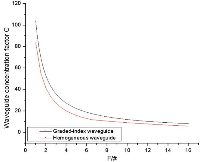
Fig. 2. Concentration factor for various  $F/\#$  of the cylindrical lens for the GRIN and the homogeneous planar solar concentrator. The chosen value for the parameter  $k$  is 2. The diameter of the lens  $D$  is 2 mm. The thickness of the waveguide  $y_{\max}$  is 1 mm. The index at the base of the GRIN waveguide  $n_0$  is 1.55.
