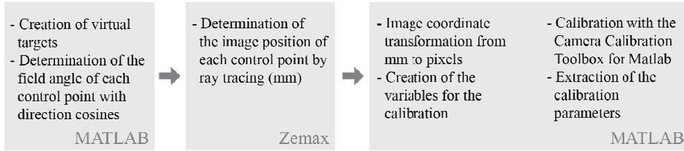
Fig. 1 Flow chart of the virtual calibration technique
