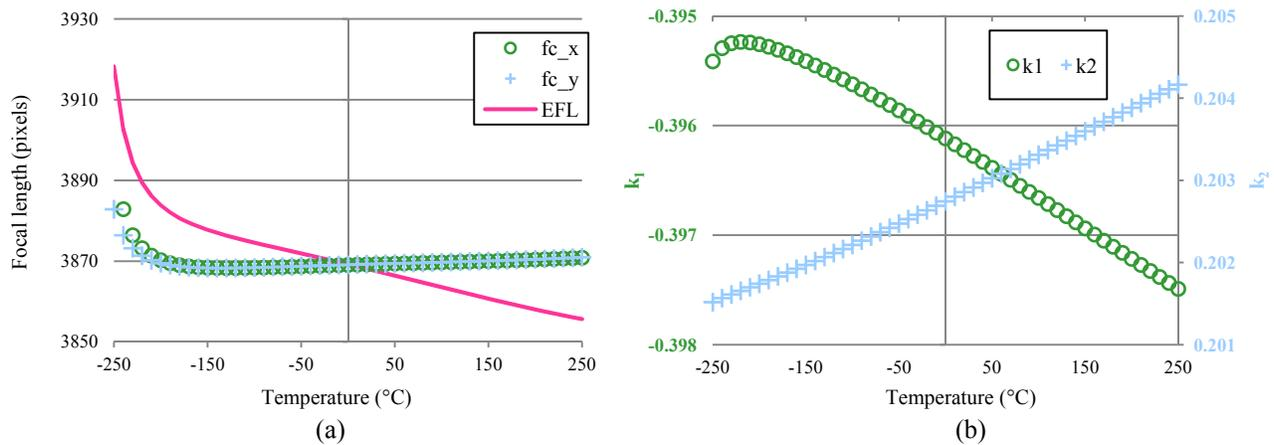
Fig. 4 (a) Calibration focal lengths and EFL obtained with Zemax® and (b) distortion coefficient  $k_1$  and  $k_2$  as a function of the temperature
