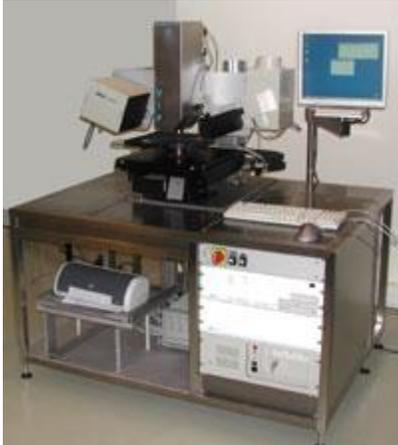
Ellipsometry measures a change in polarization as light reflects or transmits from a material structure. Ellipsometry is primarily used to determine film thickness and optical constants. However, it is also applied to characterize composition, crystallinity, roughness, doping concentration, and other material properties associated with a change in optical response.
