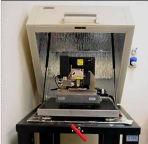
Atomic Force Microscopy (AFM) provides the ability to image the surface topography of both conducting and insulating samples, as well as adsorbed molecules and nanoparticles.
