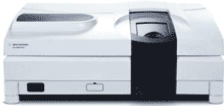
The Cary 5000 is a high performance UV-Vis-NIR spectrophotometer with superb photometric performance in the 175-3300 nm range. It measures beyond 8.0 absorbance units with reference beam attenuation using Schwarzschild coupling optics for higher accuracy at low transmission levels ensuring Maximum light throughput.
