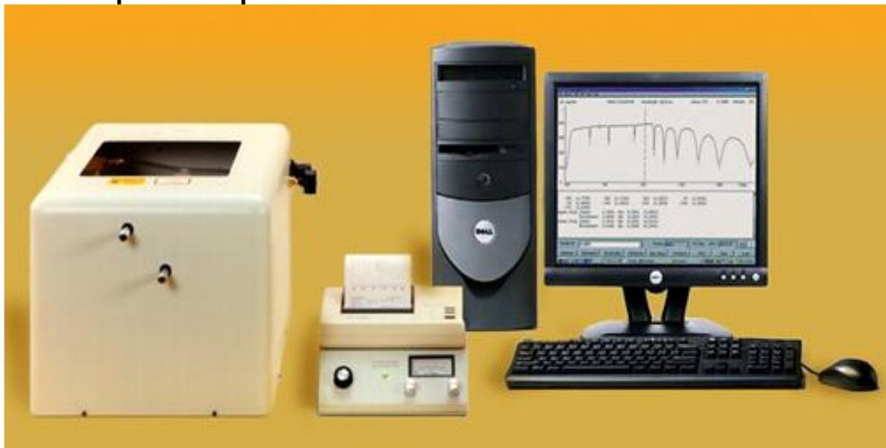
It uses optical waveguiding techniques to rapidly and accurately measure both the thickness and the refractive index/birefringence of dielectric and polymer films as well as refractive index of bulk materials. Operating at wavelengths 532, 633, 972, 1038 and 1538 nm.
