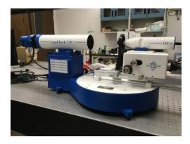
Measurement of MTF (on/off axis), EFL, F/#, BFL, astigmatism, field curvature and distortion.
