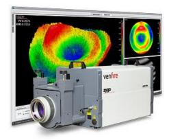
Fizeau interferometer with digital camera providing 2304 X 2304 pixels.
