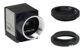
General purpose Shack-Hartmann for wavefront sensing with a  $10 \times 10$  microlens grid with a pitch of 150 um and an aperture of  $11.34 \times 7.13 \text{ mm}$ .
