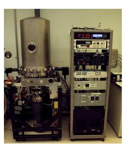
4 pockets of 7cubic centimeter to evaporate 4 different materials
