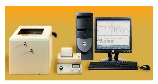
It uses optical waveguiding techniques to rapidly and accurately measure both the thickness and the refractive index/birefringence of dielectric and polymer films as well as refractive index of bulk materials. Operating at wavelengths 532, 633, 972, 1038 and 1538 nm.
